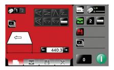
Using the screen is simplicity itself. Key in the sheet length (popular sizes are pre-set), touch the fold type for the finished product (letter, gate etc) and press the green button. The AutoCreaser Pro 50 will automatically
